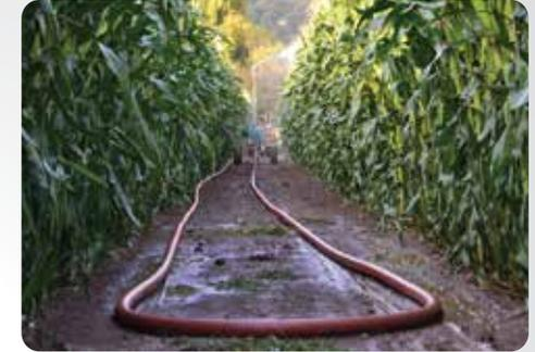
Irriforce is an irrigation machine designed for Energy Efficiency. Its cost in terms of both use and investment is lower than those of its rivals. We may call Irriforces as traveling rain gun. Thanks to water turbine and steel rope in it, it irrigates your field by dragging itself.
